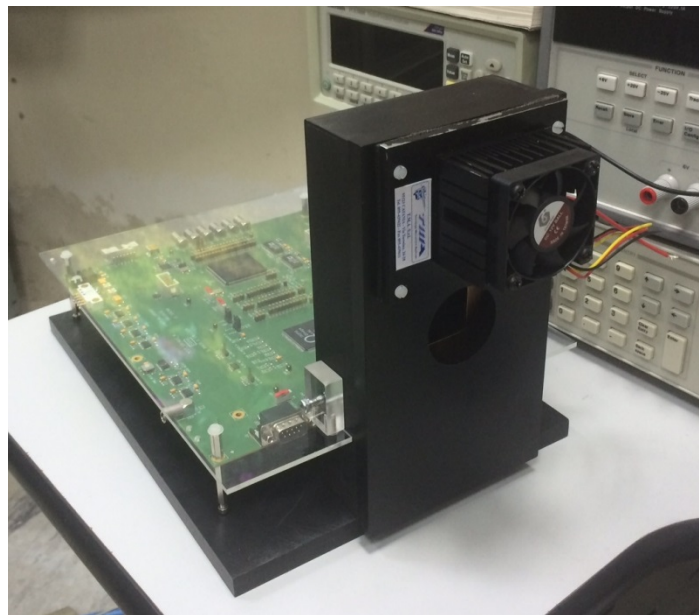
Figure 2. Citiroc evaluation board and the black light-tight box with cooling system based on Peltier TEC.
